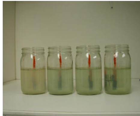
Oil reduction achieved after 48 hours of incubation. Notice the progressively better water clarity as the microbial population increases.
